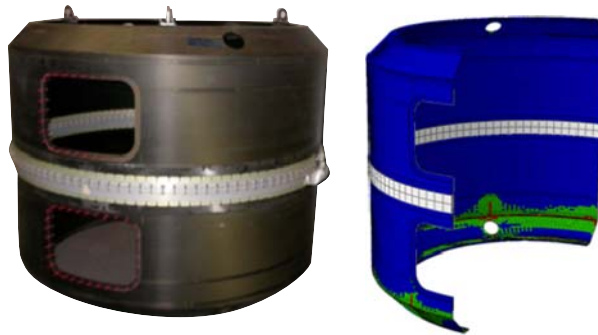
The Composite Adapter for Shared Payloads (CASPAR) and its simulation with Helius:MCT in Abaqus/Standard.
