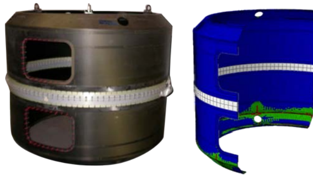
The composite Adapter for Shared Payloads (CASPAR) and its simulation with Helius:MCT in Abaqus.
