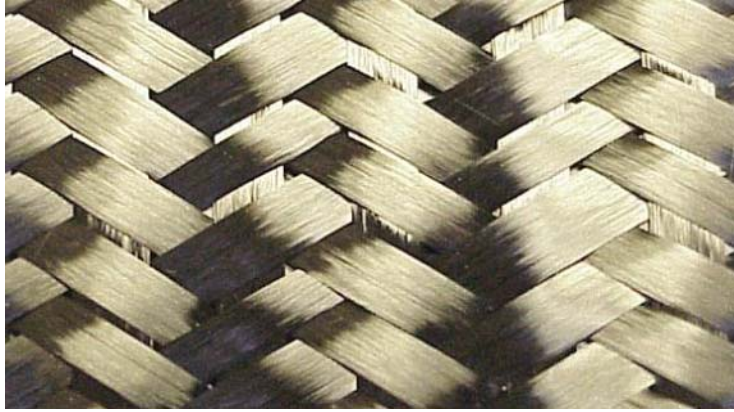
Figure 1. Triaxial carbon fiber braid with 60° yarns. (Reprinted with permission from S. P. Lomov, copyright (2010) by S. P. Lomov.)
